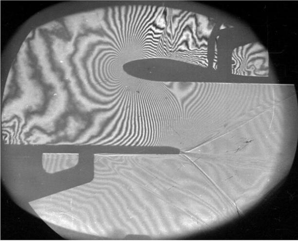
FIGURE 10. Section near the tip,  $\iota = -6.5^\circ$ ,  $M_{2is} = 1.51$ .
