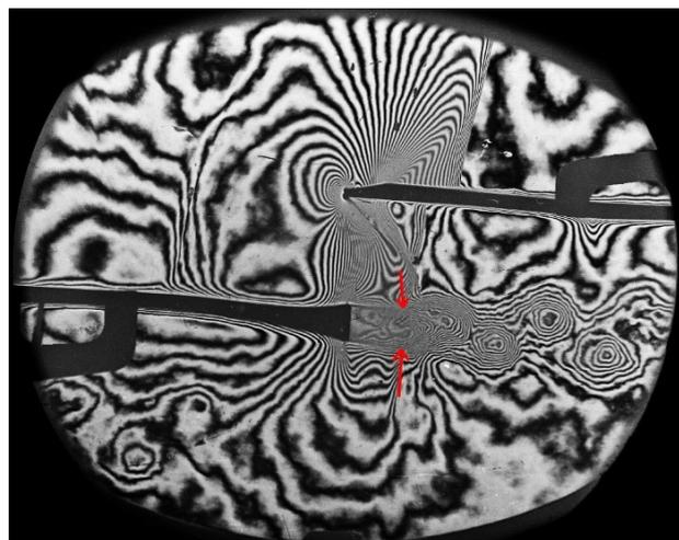
FIGURE 13. Tip section consisting of profiles with the tailored trailing edge, off-design condition of flow  $M_{2is} = 0.912$  [4].
