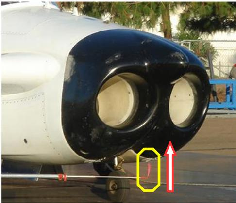
Figure 20: Prevailing flow at ground level no flow deflector
